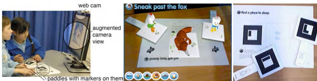
Figure 1. Left to right: Setup. On-screen scene, 3D animations over markers. Page and Paddles.
