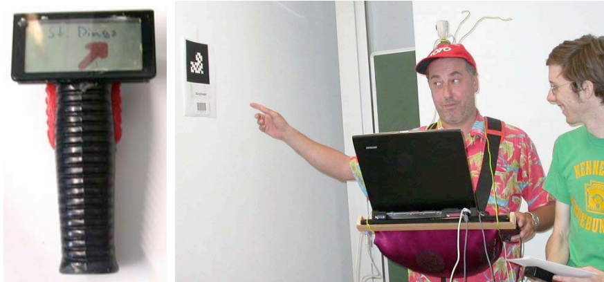
Fig. 2. Tourist Navigation Device: Mock-Up with display and vibrating (red) parts on the sides. Demo of working prototype - the system detects a visual marker (camera worn on hat) of a site and spoken text output is triggered.
