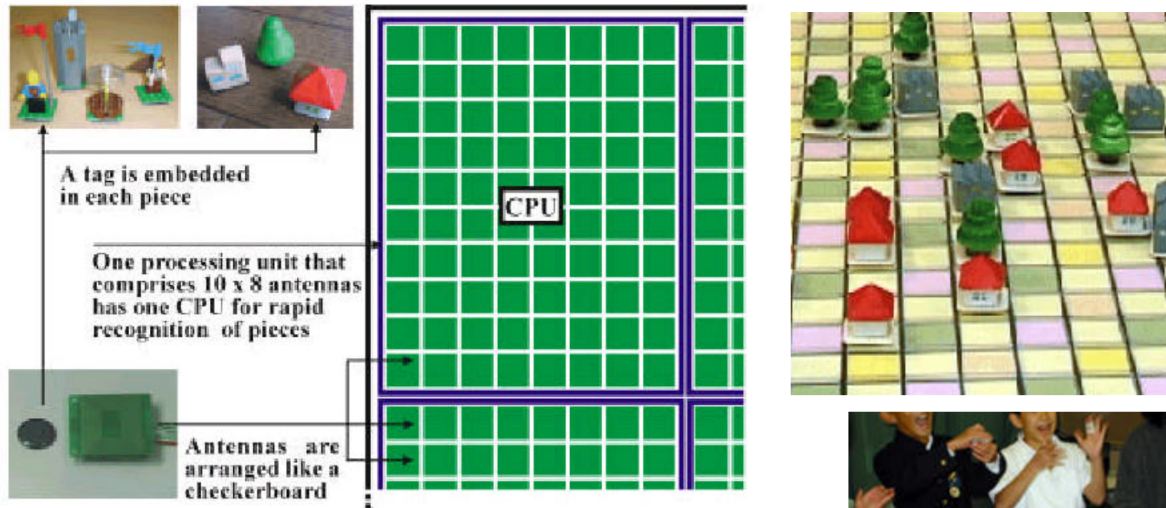
Figure 2. How RFID technology is used in E 2 board and its applications
