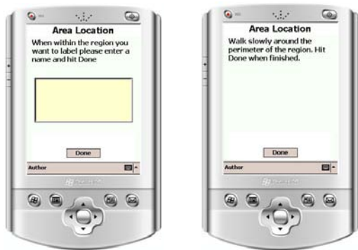
Figure 6: Defining location by walking a perimeter.
