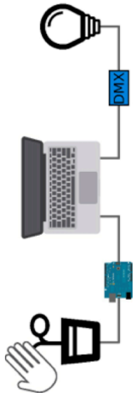
Figure 5: Overview of the implementation. Touch recognition via capacitive sensing is processed on a laptop in order to control the lights.
