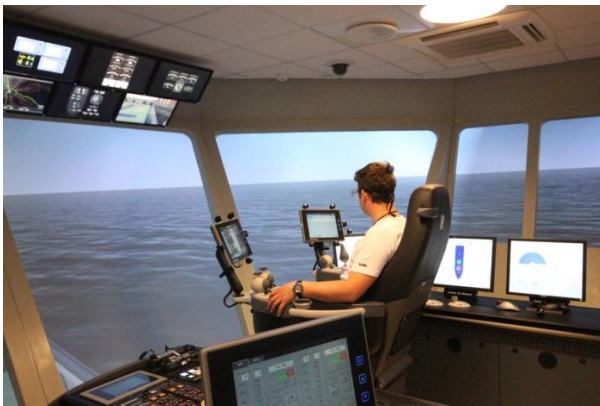
Figure 2: Simulator setting with operator using eye-tracking glasses and IR markers for marking AOIs
